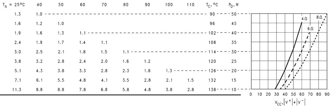
Note: The maximum heat sink thermal resistance values,  $\theta_{SA}$ , in the table above were calculated using a  $\theta_{CS} = 0.2^\circ\text{C/W}$  due to thermal compound.
