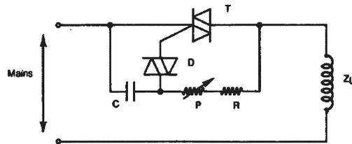
Synchronization across the triac based on crossing of the zero point by the current.
