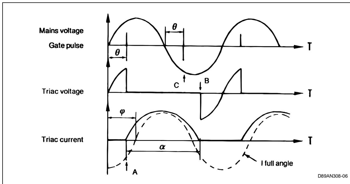
To prevent this fault, it is necessary to insert a "stop" to maintain  $\theta > \varphi$ . This is possible for loads whose L and R parameters remain strictly constant.
