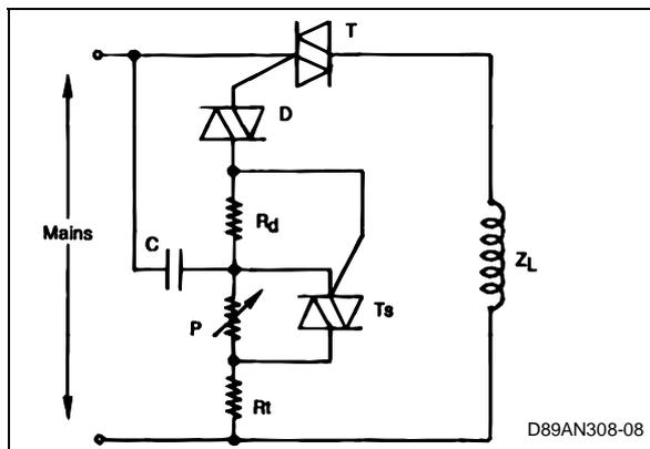
Figure 8 gives the circuit diagram. A small sensitive auxiliary triac is used to produce the pulse train necessary for maintaining the control signal.
