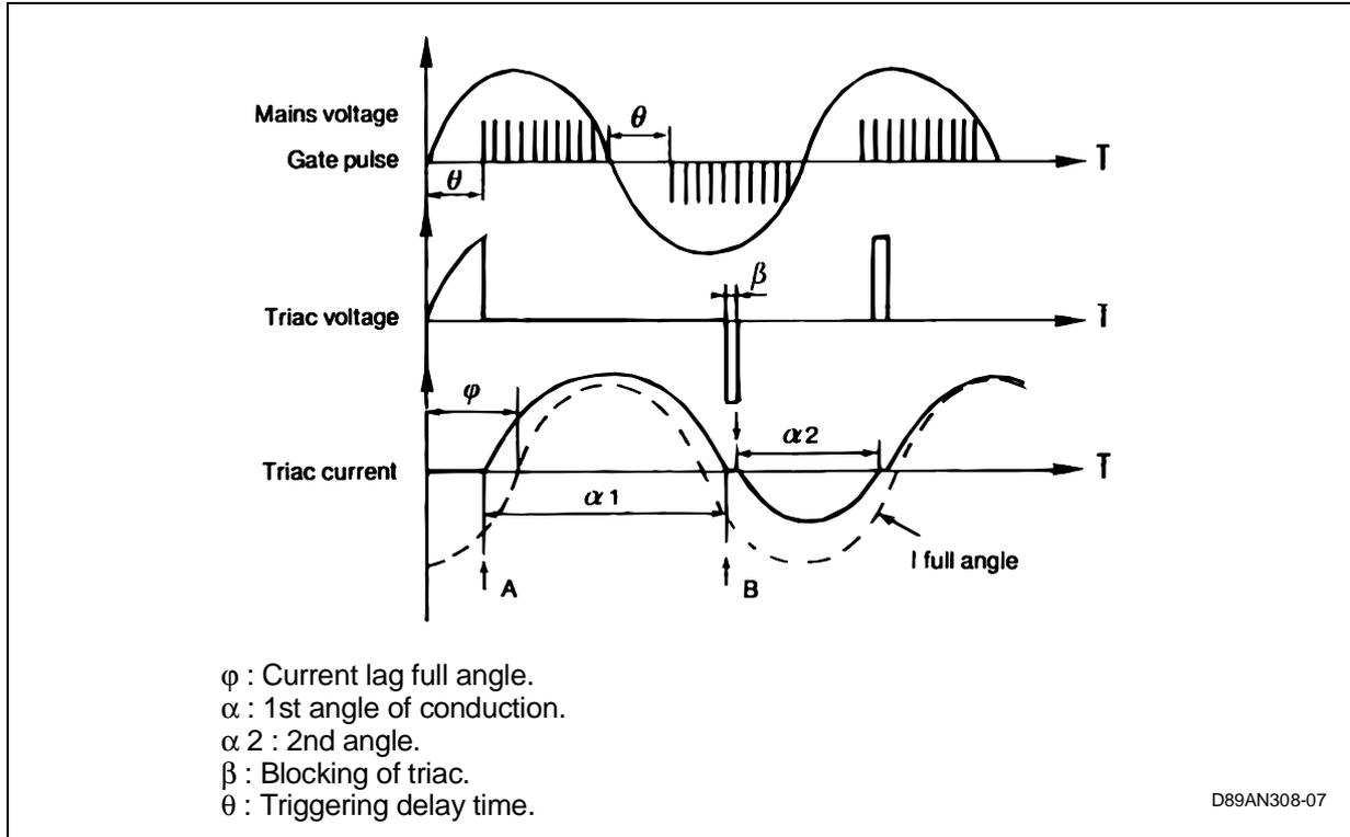
For example, suppose that angle  $\phi$  is equal to  $85^\circ$  and  $\theta$  is equal to  $60^\circ$ . At the first pulse, the triac is turned on at point A ( $60^\circ$ ). It conducts for angle  $\alpha 1$  greater than  $180^\circ$  and close to  $240^\circ$ . It is blocked at point B but is immediately triggered at point B' by the
