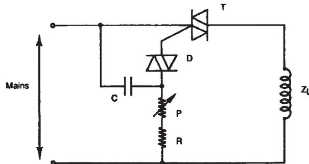
Synchronization based on crossing of the zero point by the mains voltage
