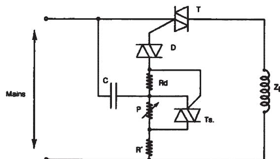
Synchronization by crossing of the zero point by the mains voltage and generation of a pulse train from then onwards.
