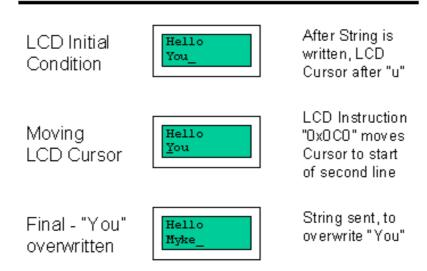
The LCD can be thought of as a "Teletype" display because in normal operation, after a character has been sent to the LCD, the internal "Cursor" is moved one character to the right. The "Clear Display" and "Return Cursor and LCD to Home Position" instructions are used to reset the Cursor's position to the top right character on the display.
