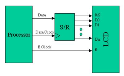
This can be further reduced by using the circuit shown below in which the serial data is combined with the contents of the shift register to produce the "E" strobe at the appropriate interval.
