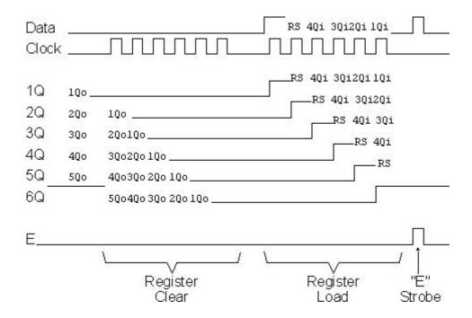
I normally use a 74LS174 wired as a shift register (as is shown in the schematic diagram) instead of a serial-in/parallel-out shift register. This circuit should work without any problems with a dedicated serial-in/parallel-out shift register chip, but the timings/clock polarities may be different. When the 74LS174 is used, note that the data is latched on the rising (from logic "low" to "high") edge of the clock signal.
