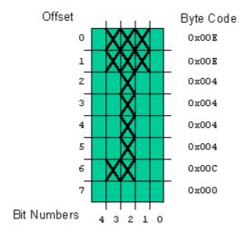
The user defined character line information is saved in the LCD's "CGRAM" area. This sixty four bytes of memory is accessed using the "Move Cursor into CGRAM" instruction in a similar manner to that of moving the cursor to a specific address in the memory with one important difference.
