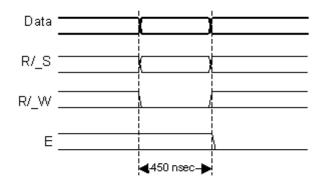
This waveform will write an ASCII Byte out to the LCD's screen. The ASCII code to be displayed is eight bits long and is sent to the LCD either four or eight bits at a time. If four bit mode is used, two "nybbles" of data (Sent high four bits and then low four bits with an "E" Clock pulse with each nybble) are sent to make up a full eight bit transfer. The "E" Clock is used to initiate the data transfer within the LCD.
