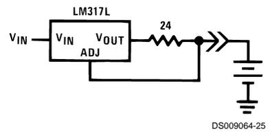
5V Logic Regulator with Electronic Shutdown\*
