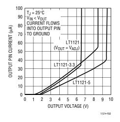
Figure 2. Reverse Output Current
