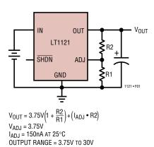
Figure 1. Adjustable Operation
