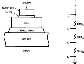
Figure10. MOSFET Steady-State Thermal Resistance Model
