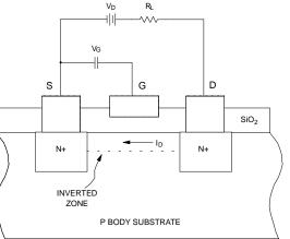
Figure 1. Lateral N-Channel MOSFET Cross-Section
