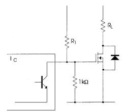
Figure 20. Open Collector TTL Drive Circuit
