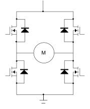
Figure 5. Full-Wave Motor Control Circuit
