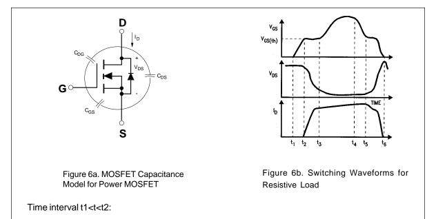
The initial turn-on delay time  $t_{d(ON)}$  is due to the length of time it takes  $V_{GS}$  to rise exponentially to the threshold voltage  $V_{GS(TH)}$ . From Figure 6, the time constant can be seen to be  $R_S x C_{GS}$ .
