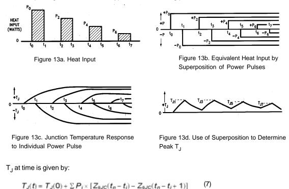
The typical use condition is to compute the peak junction temperature at thermal equilibrium for a train of equal amplitude power pulses as shown in Figure 14.
