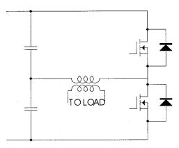
Figure 24. Half-Bridge Configuration
