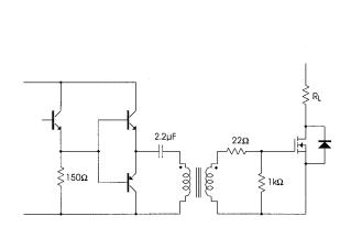
Figure 27. Emitter Follower Driver with Speed-Up Capacitor
