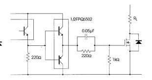
Figure 22. Circuit for PWM IC Driving MOSFET. The PNP Transistor Speeds Up Turn-Off
