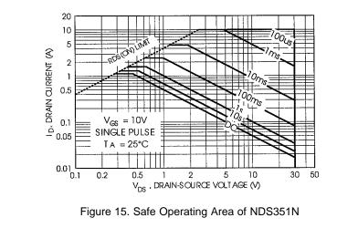
Note that the safe area boundaries are only thermally limited and exhibit no derating for second breakdown. This shows that while the MOSFET transistor is very rugged, it may still be destroyed thermally by forcing it to dissipate too much power.
