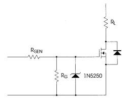
Figure 28. Zener Diode to Prevent Excessive Gate-Source Voltages
