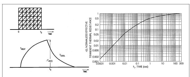
Figure 12a. Junction Temperature Response to a Step Pulse of Heating Power
