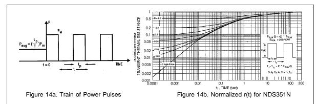
To further simplify this calculation, the bracketed expression in equation (G) has been plotted for all Fairchild Semiconductor Power MOSFETs, as exemplified by the plot of  $Z_{\theta JC}$  in Figure 14b. From this curve, one can readily calculate  $T_J$  if one knows  $P_M$ .  $Z_{\theta JC}$  and  $T_C$  using the expression:
