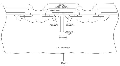
Figure 3. Vertical DMOS Cross-Sectional
