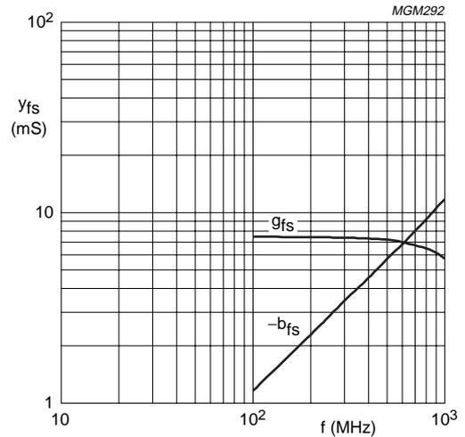
$V_{DS} = 15\text{ V}; V_{GS} = 0; T_{amb} = 25\text{ }^{\circ}\text{C}.$
