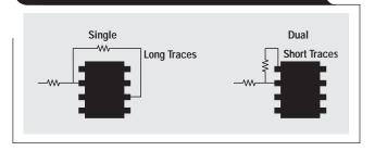
The single op amp package places the output on the opposite side from the inputs. This can be a disadvantage at high speeds because it forces longer PCB traces. It may make more sense to use a dual op amp package, even if the second op amp is unused. Figure 10 illustrates trace length for an inverting op amp stage.
