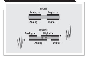
Figure 2. Single ground point minimizes ground loops
