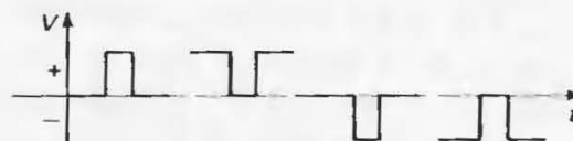
Figure 1.25. Positive- and negative-going pulses of both polarities.
