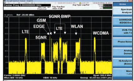
5G NR must coexist with the many already existing services and with new services that will be introduced to support 5G use cases. Different signals can be found in adjacent and in non-contiguous spectrum, making interference a big issue. To reduce adjacent spectrum interference, in-band and out-of-band emissions must be minimized.
