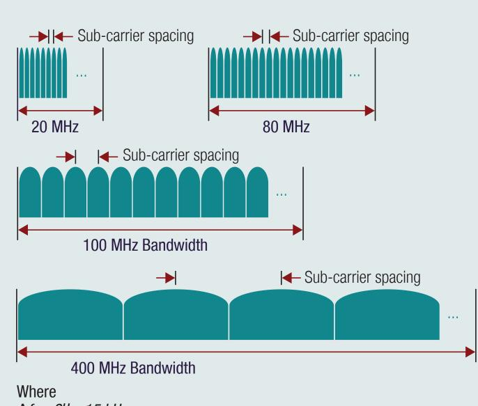
$\Delta f = 2\mu x 15 \text{ kHz}$ Example: 15 kHz, 30 kHz, 60 kHz ... 480 kHz subcarrier spacing
