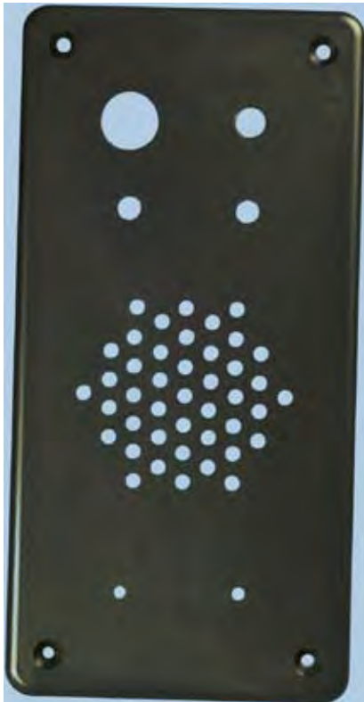
Figure 3-108. The exterior of the panel after drilling. A small handheld cordless drill can create a neat result if the holes were marked carefully.
