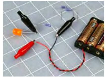
Figure 1-44. The setup for Experiment 3, showing resistors of 470\Omega , 1K\Omega , and 2K\Omega . Apply alligator clips where shown, to make a secure contact, and try each of the resistors one at a time at the same point in the circuit, while watching the LED.
