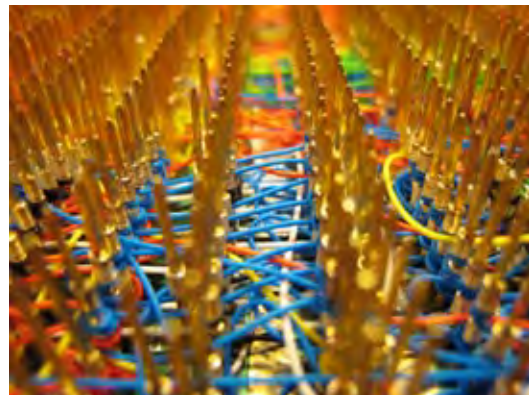
Figure 3-37. This picture shows some of the wire-wrapping in Steve Chamberlin's custom-built, retro 8-bit CPU and computer. “Back in the day,” connecting such a network of wires with solder joints would have been unduly time-consuming and prone to faults. Photo credit: Steve Chamberlin.
