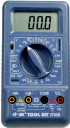
Figure 1-5. You can see by the wear and tear that this is my own favorite meter. It has all the necessary basic features and can also measure capacitance (the F section, for Farads). It can also check transistors. You have to choose the ranges manually.
