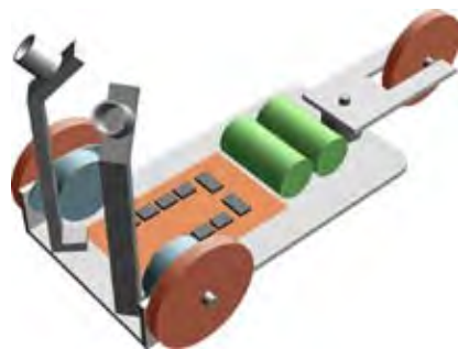
Figure 5-121. This 3D rendering shows a possible configuration of the light-seeking cart, with two photoresistors enclosed in small tubes to restrict their response to light.
