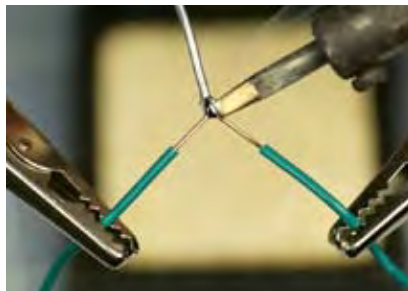
Figure 3-35. This and the preceding three figures illustrate four steps to making a solder joint: apply heat to the wires, bring in the solder while maintaining the heat, wait for the solder to start to melt, and wait a moment longer for it to form a completely molten bead. The whole process should take between 4 and 6 seconds.
