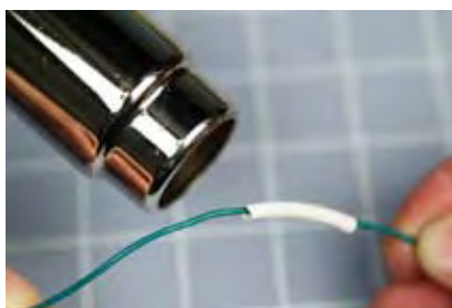
Figure 3-49. Apply heat to the tubing.
