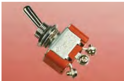
Figure 2-12. This relatively large toggle switch made by NKK has screw terminals, which will reduce the inconvenience of attaching it to hookup wire.
