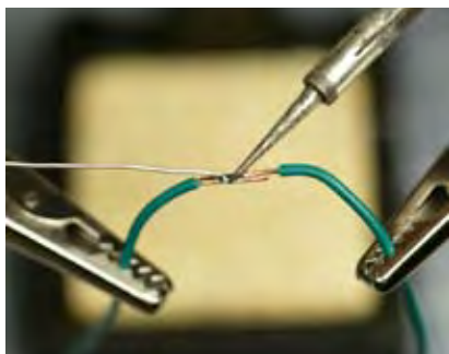
Figure 3-43. This and the preceding three figures show how joining two wires that are parallel is more difficult, and the low-wattage, pencil-type soldering iron will require longer to heat them sufficiently for a good joint. Thinner solder can be used.
