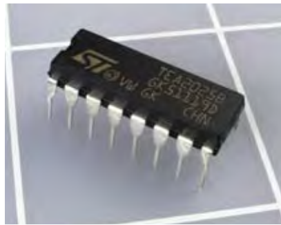
Figure 5-36. This single chip contains a stereo amplifier capable of delivering a total of 5 watts into an 8\Omega speaker when the two channels are combined.
