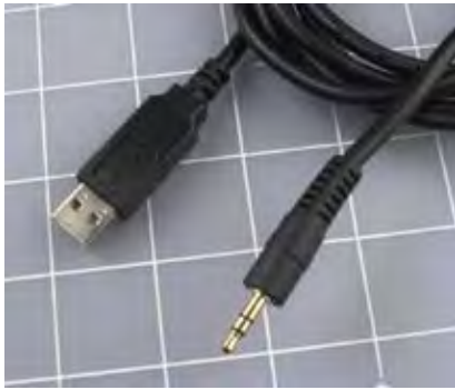
Figure 5-125. The USB download cable made for use with the PICAXE terminates in a 3.5-mm audio plug. This should not be inserted in any audio device. It establishes a serial connection with a computer, allowing program code to be downloaded into the chip.
