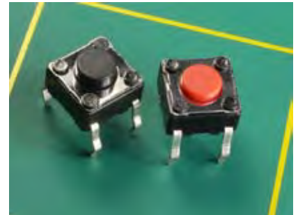
Figure 4-9. A tactile switch delivers tactile feedback through your fingertip when you press it. They are almost always SPST pushbuttons designed for mounting in circuit boards with standard 1/10-inch hole spacing.
