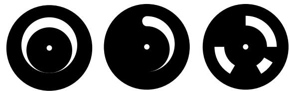
Figure 5-58. Different stripe patterns could be used in conjunction with the imaginary electromechanical device in Figure 5-57 to create various tremolo effects.
