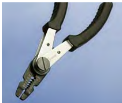
Figure 2-4. To use these wire strippers, insert a piece of insulated wire in the appropriate-sized hole between the jaws, grip the handles, and pull a section of insulation away. See page 45.
