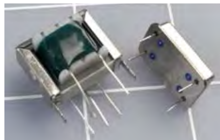
Figure 5-73. An AM radio transmitter can be made from just two components: a transformer (left) and a crystal oscillator (right), available from http://www.scitoys.com .
