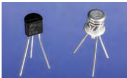
Figure 2-13. Transistors are commonly sold either in little metal cans or sealed into little lumps of plastic. For our purposes, the packaging makes no difference.
