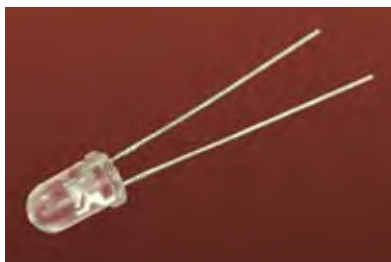
Figure 1-14. Typical 5-mm diameter light-emitting diode (LED).
