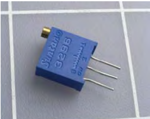
Figure 5-117. Close-up of a trimmer potentiometer with pins spaced at 1/10 inch for insertion in a breadboard or perforated board. The brass screw, at top-left, turns a worm gear inside the unit, allowing precise adjustment of internal resistance.
