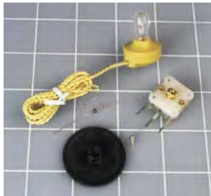
Figure 5-59. Just add wire and a coil, and this is all you need to receive AM radio signals. The black disc becomes the tuning dial, after it is screwed onto the variable capacitor (right). This is actually an optional extra. A germanium diode (center) rectifies the radio signal. The high-impedance earphone (top) creates a barely audible sound.
